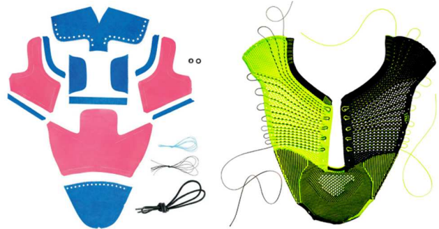
Fig. 3. Components of a traditional shoe upper (left) [21] and a Flyknit upper (right) [22]
