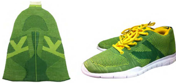
Fig. 2. Flat-knitted upper developed by Lu [6]
