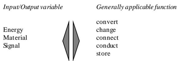
Fig. 3. Definition of generally applicable functions [20]
