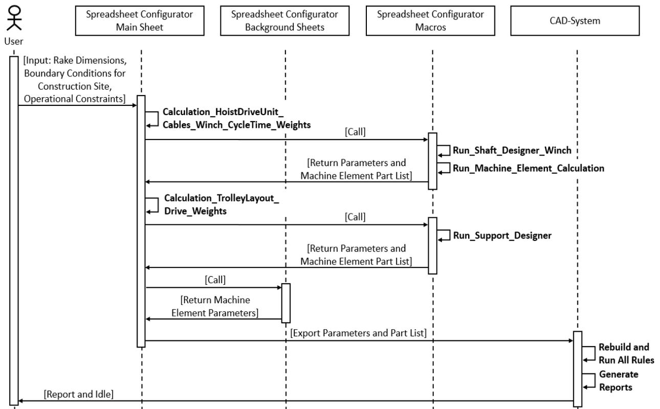
Fig. 8. Sequence Diagram for Trash Rack Cleaner Configuration
