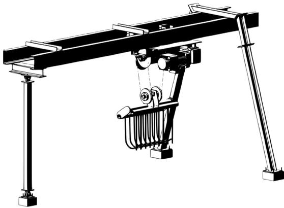
Fig. 3. *Cable Trash Rack Cleaner with Gripper Head*
