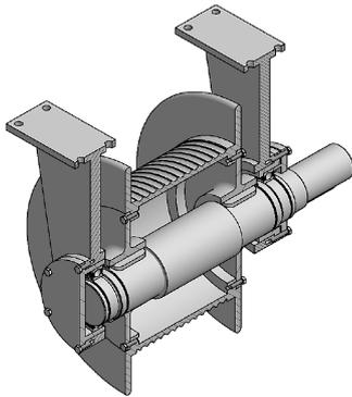
Fig. 5. Cable Drum (Sectional View)
