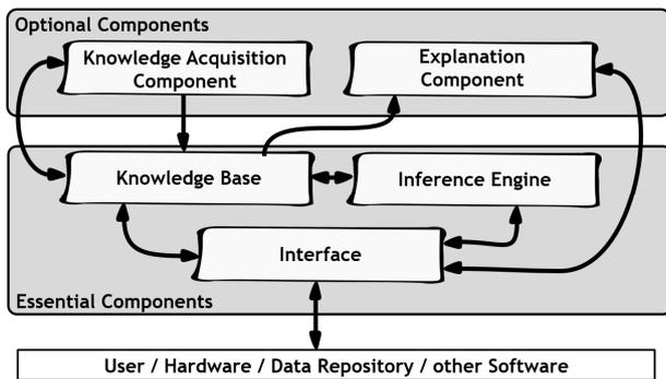
Fig. 1. Main Components of a Knowledge-Based System (acc. to [8])
