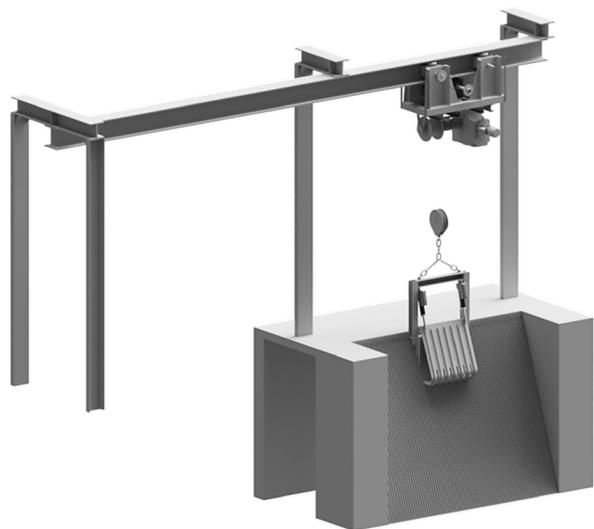
Fig. 9: Configured Trash Rack Cleaning System (Illustration without Cables, Casing, Foundations, Top Plates and Screw Connections)
