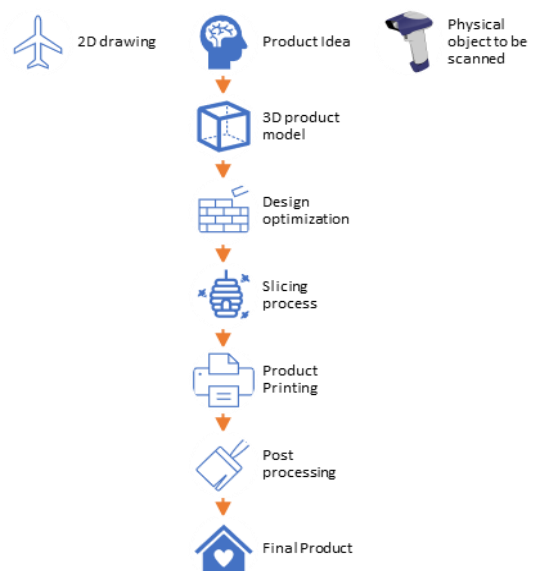
Fig. 3. AM process flow
