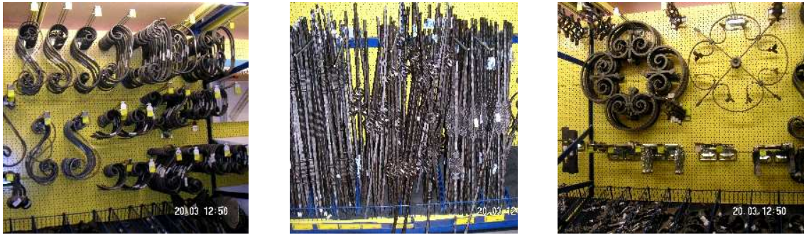
Figure 7 Mass produced elements made with forging machies
