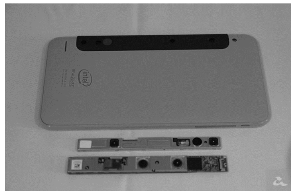
Fig. 10. Intel RealSense 3D cameras and their place on the smartphones –
