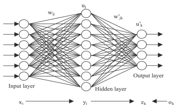
Fig. 1. Basic construction of the simple feed-forward ANN, Source [17]
