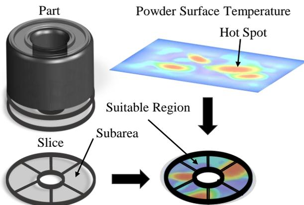
Fig. 6. Generation of geometry-dependent subareas
