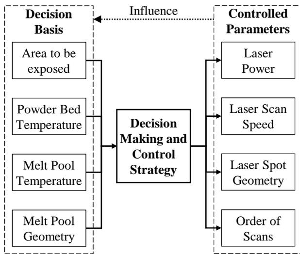
Fig. 5. Basis for the control strategy and controlled parameters
