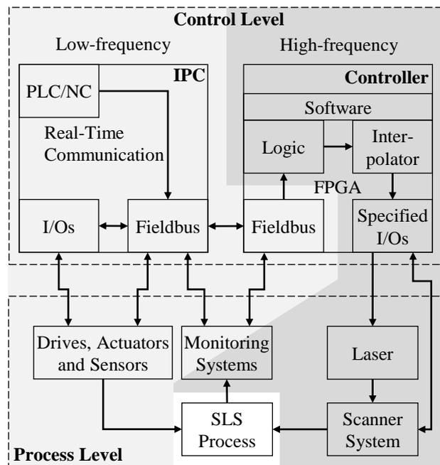
Fig. 4. Schematic diagram of control platforms for laser-based processes using FPGA
