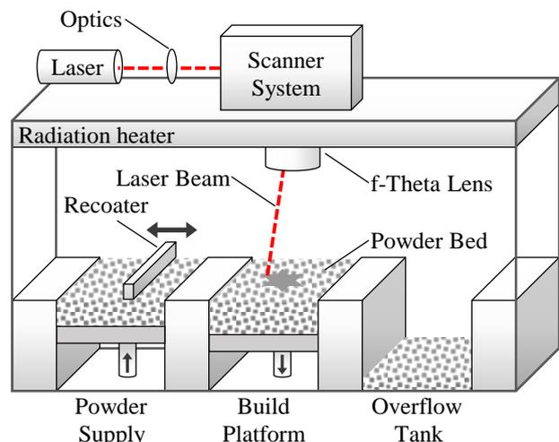
Fig. 1. Schematic diagram of Selective Laser Sintering
