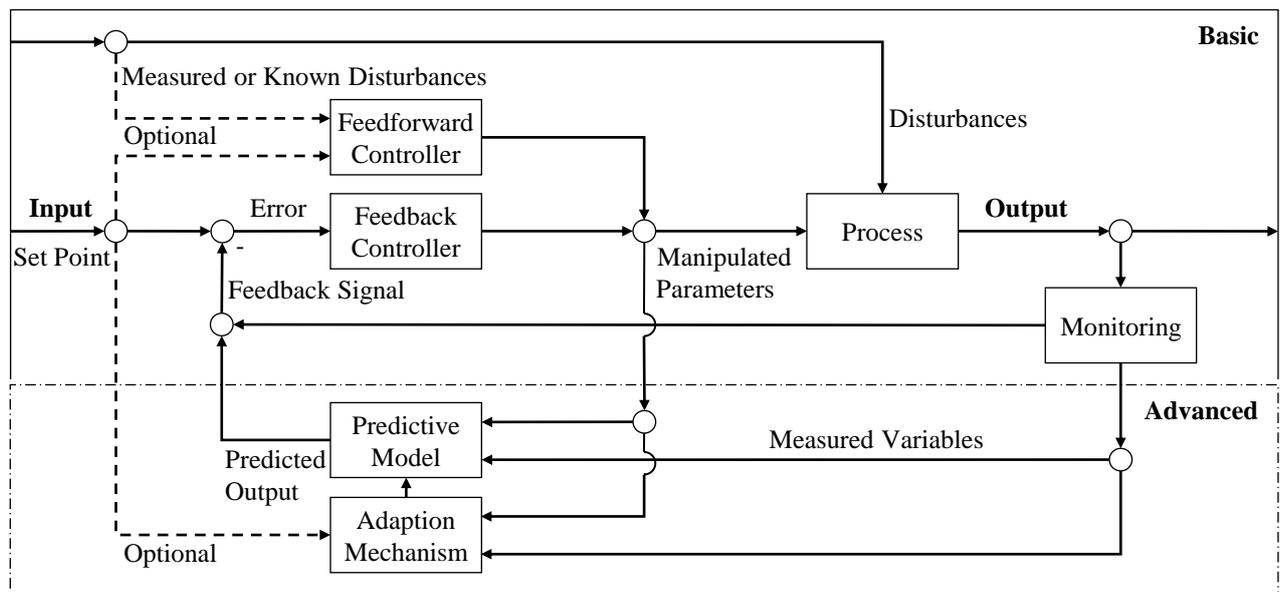
Fig. 3. Simplified control architecture with feedback, feedforward and adaptive model predictive control
