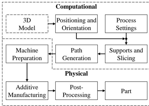
Fig. 2. Process chain for Additive Manufacturing
