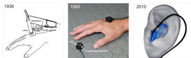
Fig. 1. Progress in photoplethysmography and its sensor concepts: First optoelectronic sensor by Hertzman [5] with incandescent lamp as polychromatic light source and selenium cell as photo detector (left); an universal reflective PPG sensor on the market today (middle); and novel personalized in-ear rPPG sensor (right).
