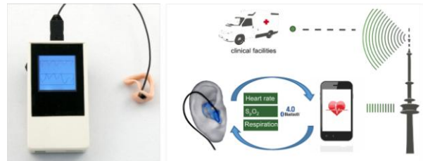
Fig. 5. Function diagram of the in-ear PPG monitoring system strategy - as a single device (left) or as a system part of a medical support monitoring chain (right).
