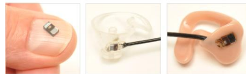
Fig. 4. Different in-ear PPG sensor prototypes, developed at the RWTH Aachen University. The silicon chip containing both the light emitters and the photo-receiver (CiS Erfurt, Germany) is assembled on a flexprint board (left), universal in-ear sensor module (available in different size, middle), individually customized/personalized sensor module (right).
